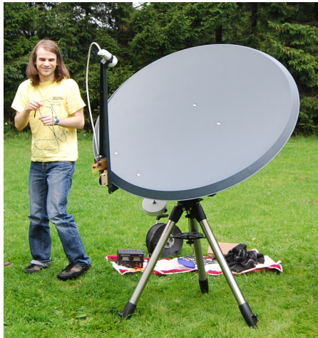
Figure 2: Left image: The complete telescope, with mount, LNB and electronics (and me). Right image: Detail photo of how the dish is fixed on the mount.
