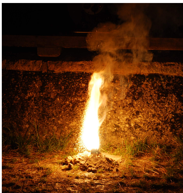
Figure 9: The first try to detect a thermite reaction (50 g of substrate) with the radio telescope, the receiver being outside of the imaged area in this case. In a second try, after the flame went out, the receiver was put directly above the remaining hot iron to make it fill a larger part of the solid angle observed by the receiver. The reflector dish was not used for this experiment.
