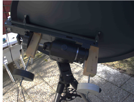
Figure 2: Left image: The complete telescope, with mount, LNB and electronics (and me). Right image: Detail photo of how the dish is fixed on the mount.
